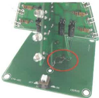
13. Wires pass through the holes and cut off the excess wires.
