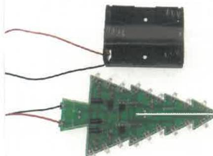
Install and test B board
