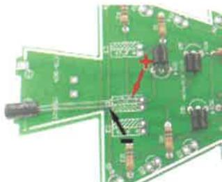
4. Install Electrolytic capacitor
